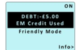
This screen shows that all of the Emergency credit has been used and the **'DEBT'** is now **'-£5.00'**. The supply is now **'OFF'** and will only be reconnected once the **'DEBT'** has been repaid in full.
